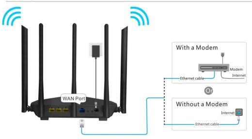
4. Connect your wireless device such as a smart phone to the new router's WiFi network using the WiFi name and password on the top / bottom label.
