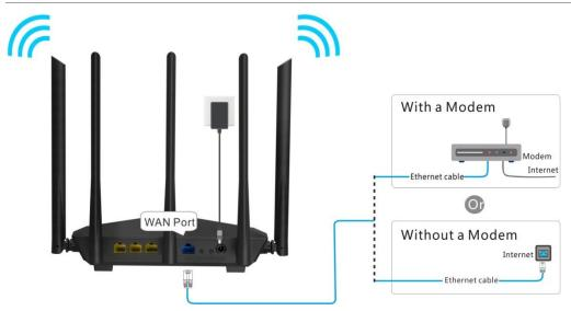
**4.** Connect your computer to port 1, 2 or 3/IPTV of the router using an Ethernet cable.
